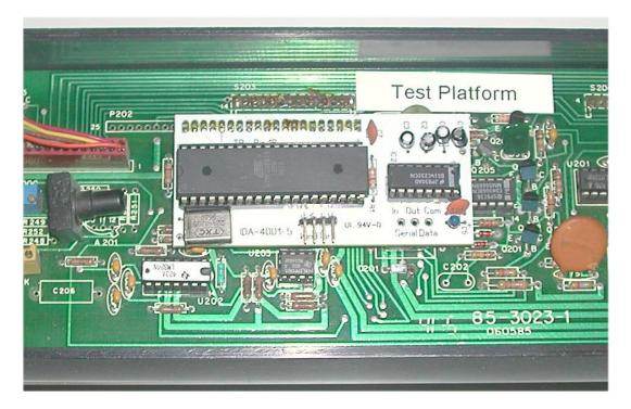
Make certain the all 40 pins from the adapter board are firmly inserted into the corresponding 40 pins of the original IC socket.
